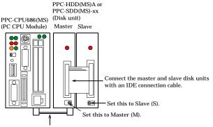
Connect the PC CPU Unit to the master disk unit with an IDE connection cable.
